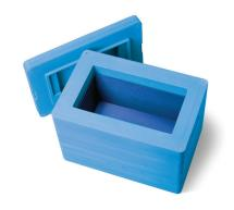
**BioT** LN2 Transporter is comprised of five parts: magnetized lid, thermo-conductive basket, thermo-conductive shelf plate, absorbent/baffle pad and base chamber. To begin simply insert the thermo-conductive basket into empty base chamber, followed by the absorbent/baffle pad. Place the thermo-conductive shelf plate into the basket on top of the absorbent/baffle pad. With the addition of LN2, (~ 2.7L) the internal chamber will reach <-150°C within approximately 10 minutes.
