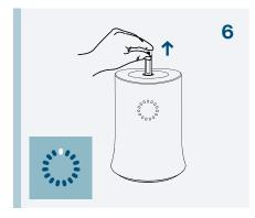
Remove vial immediately and for a few seconds, manually agitate the vial gently from side to side to equilibrate the liquid temperature until no ice can be seen within the vial. Begin downstream protocol.
