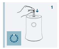
Unit is warmed up and in "ready" state. Insert a clean, tightly capped frozen 1.5 mL cryogenic vial (below -70°C) containing up to 1.5 mL volume into the opening on the top of the unit.
