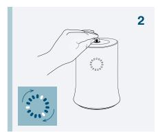
Push the top of the vial down gently until the unit emits a deep dual tone. The vial will now remain in a depressed position.
