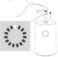
Remove vial immediately and for a few seconds, manually agitate the vial gently from side to side to equilibrate the liquid temperature until no ice can be seen within the vial. Begin downstream protocol.
