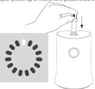
Instrument is warmed up and in "ready" state. Insert a clean, tightly capped frozen 1.5 mL cryogenic vial (below -70°C) containing up to 1.5 mL volume into the opening on the top of the instrument.
