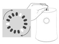
Push the top of the vial down gently until the instrument emits a deep dual tone. The vial will now remain in a depressed position.
