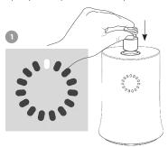
Unit is warmed up and in "ready" state. Vertically insert a clean, tightly capped frozen 6.0 mL AT-Closed Vial\* (below -70°C) containing 2.0 - 6.0 mL volume into the opening on t he top of the instrument.
