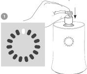
Unit is warmed up and in "ready" state. Vertically insert a clean, tightly capped frozen 2.0 mL AT-Closed Vial\* (below -70°C) into the opening on the top of the instrument.
