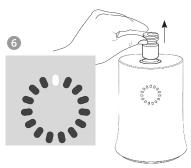
Remove vial immediately and gently swirl vial contents until remaining ice melts to equilibrate the solution to final thaw temperature.
