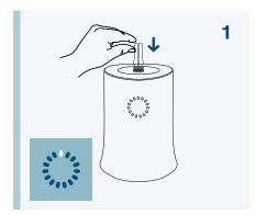
Instrument is warmed up and in "ready" state. Insert a clean, sealed frozen 5.0mL CellSeal® Cryogenic Vial (below -70°C) containing 2.5mL to 5.0mL volume into the opening on the top of the instrument.
