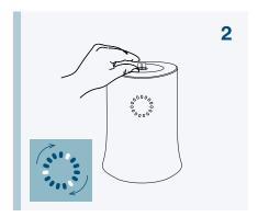
Push the top of the vial down gently until the instrument emits a deep dual tone. The vial will now remain in a depressed position.
