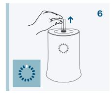
Remove vial immediately and for a few seconds, manually agitate the vial gently without inverting the vial to equilibrate the liquid temperature until no ice can be seen within the vial. Begin downstream protocol.
