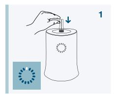
Instrument is warmed up and in "ready" state. Insert a clean, sealed frozen 2.0mL CellSeal® Cryogenic Vial (below -70°C) containing 1.0mL to 2.0mL volume into the opening on the top of the instrument.
