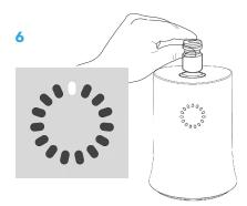
Remove vial immediately and gently swirl vial contents until remaining ice melts to equilibrate the solution to final thaw temperature.
