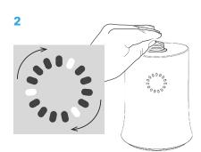
Push the top of the vial down gently until the instrument emits a deep dual tone. The via will now remain in a depressed position.
