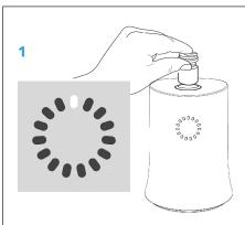
Unit is warmed up and in "ready" state. Vertically insert a clean, tightly capped frozen 2.0 mL AT Closed Vial® (below -70°C) into the opening on the top of the instrument.
