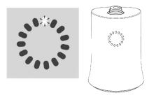
Unit begins countdown when vial load is detected. The total thaw time is calculated for the vial load detected by customized algorithms.
