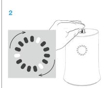
Push the top of the vial down gently until the instrument emits a deep dual tone. The vial will now remain in a depressed position.
