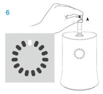
Remove vial immediately and for a few seconds, manually agitate the vial gently from side to side to equilibrate the liquid temperature until no ice can be seen within the vial. Begin downstream protocol.
